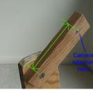
Next, cut the arm. To ligure out the length, start with that previously measured distance between the entrance pupil and the screw socket (the one that was 4 1/8 inches on my Canco) – this distance is shown in green above. Add a half inch to an inch on either side. The width need only be a couple inches.
